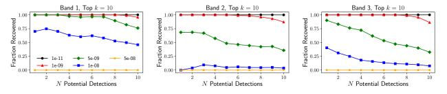
Figure 2: Results showing the average fraction of top k detection that are still recoverable as SEUs are introduced at various rates.
