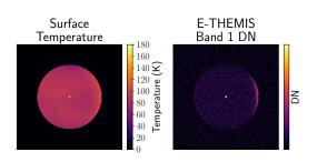
Figure 1: An example simulated E-THEMIS observation showing the instrument field-of-view in both temperature and derived DN values for Band 1 (7–14  $\mu$ m).
