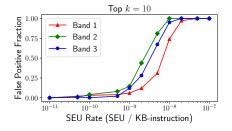
Figure 3: The fraction of false positives within the top k detections for each band as a function of SEU rate.
