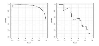
Figure 5. Precision and recall curves based on varying classifier confidence. Left: Training performance on 9P/Tempel. Right: Test performance on 103P/Hartley using the model trained on 9P/Tempel.
